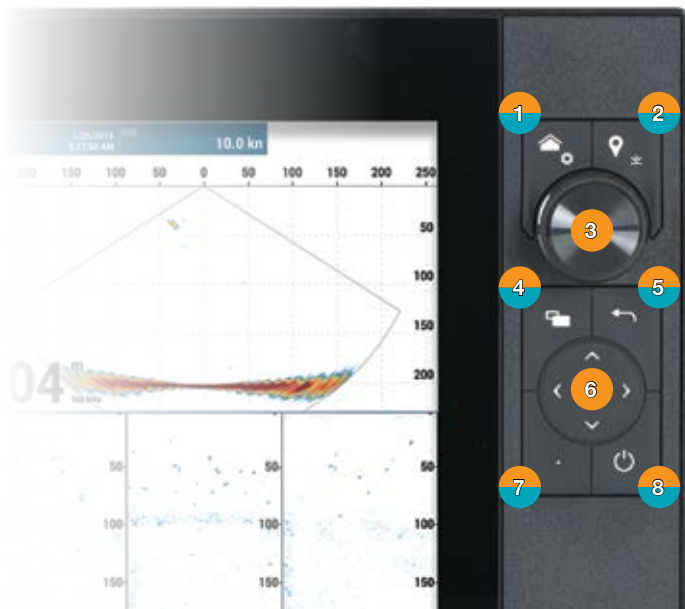
Model TZT19F - 19" >>> Spec P86 19" Multi-Touch MFD 1920x1080 (FHD) with built-in TruEcho CHIRP™ Fish Finder
