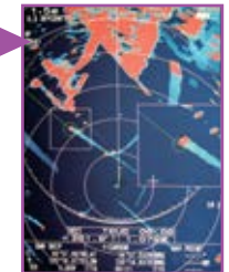
Target A3: Zoom box tracks the targeted object according to its movement
