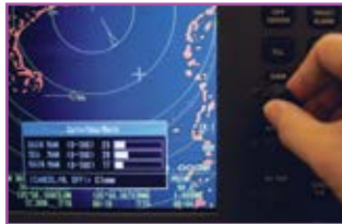
Dedicated rotary knobs to adjust GAIN/STC/FTC for simplified control.
